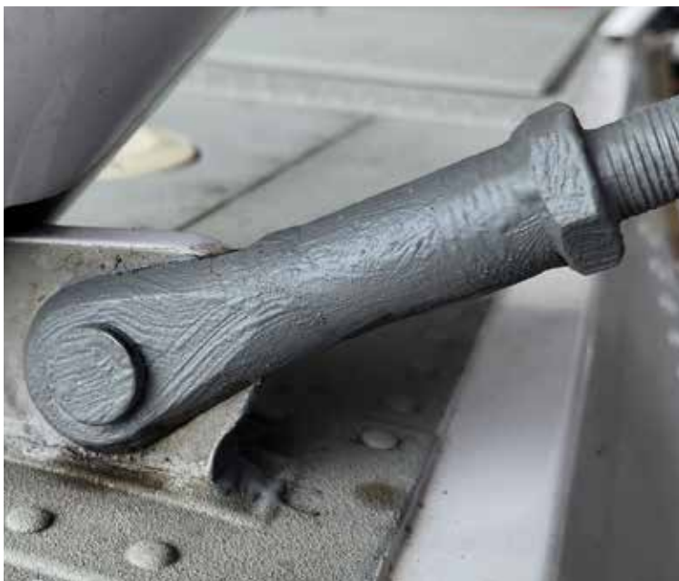
Lower flying wire attachment
