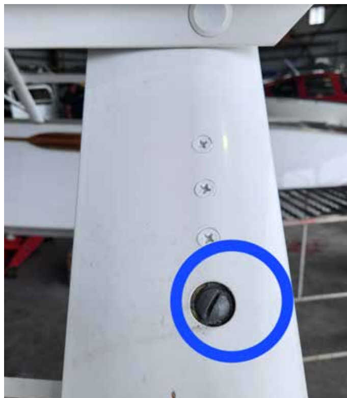
FWD support strut bolt
